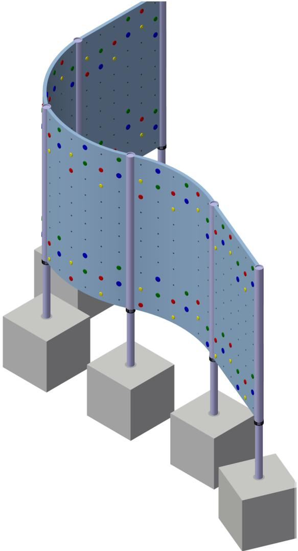
On site foundations 80 x 80 x 80 cm with internal slot for the pillars  $\text{Ø} 15 \text{ cm} \times L = 40 \text{ cm}$  in the foundations. Therefore please use the pre-supplied plastic hollow sleeve ( $\text{Ø} 15 \text{ cm}$ ). Concrete which is at least with C20/25 classification is to be used.
