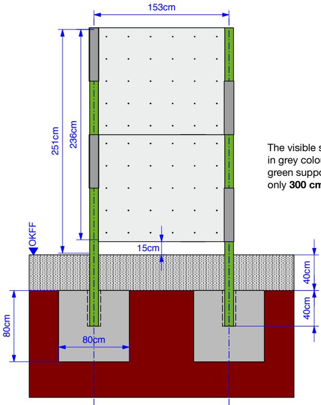
The visible sleeves are shown in grey colour. The hidden, green supporting tubes are only 300 cm long!
